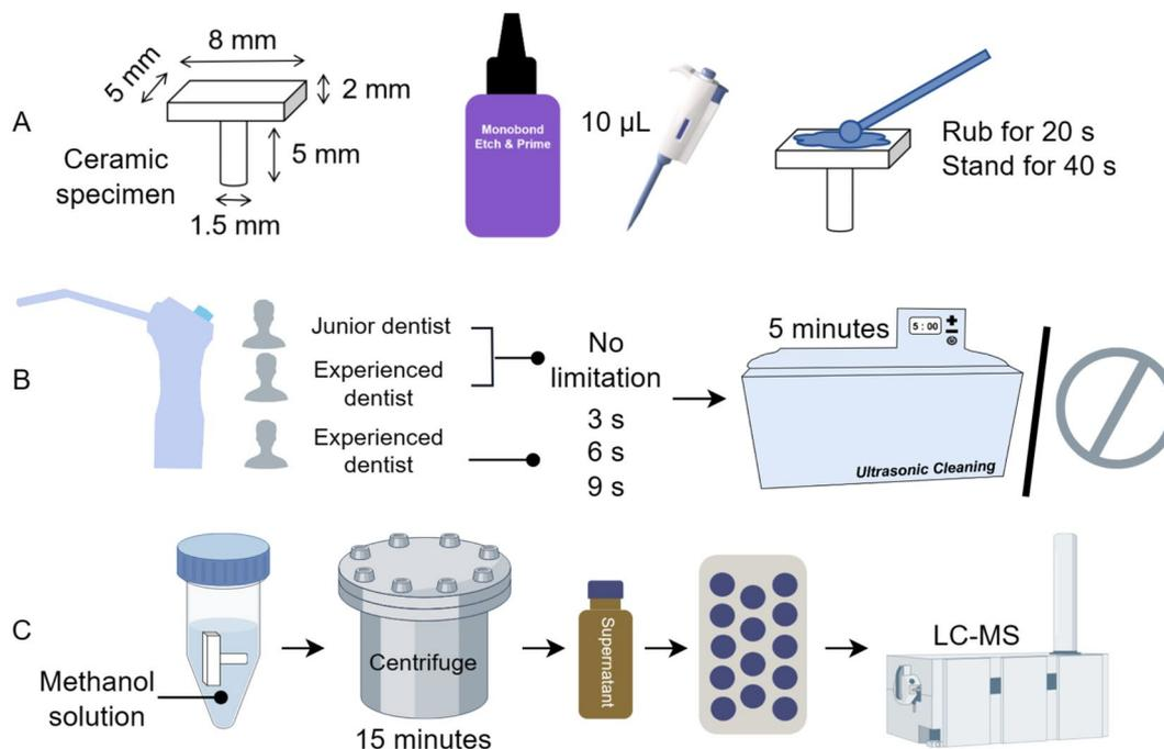
**Fig. 3** Experimental design of the study. (A, Etching. B, Flushing. C, Testing)
